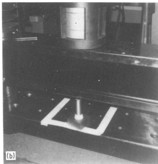
Figure 1 Potting resin/plastic material adhesion testing: (a) shows the accessory and (b) shows the actual testing on an Instron machine.
